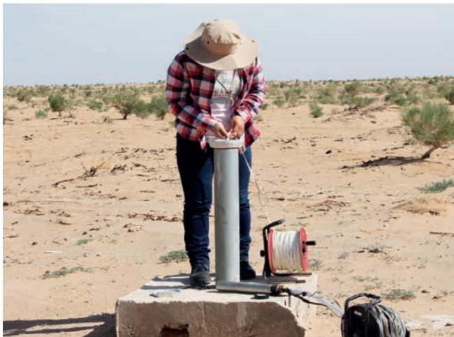
Employee measuring groundwater level in a monitoring well
